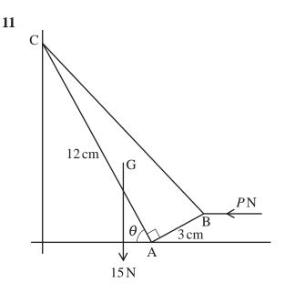
The diagram shows the cross-section through the centre of mass of a uniform solid prism. The cross-section is a right-angled triangle ABC, with AB perpendicular to AC, which lies in a vertical plane. The length of AB is 3 cm, and the length of AC is 12 cm.
