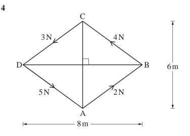
A rigid lamina of negligible mass is in the form of a rhombus ABCD, where AC = 6 m and BD = 8 m. Forces of magnitude 2N, 4N, 3N and 5N act along its sides AB, BC, CD and DA, respectively, as shown in the diagram. A further force **F**N, acting at A, and a couple of magnitude *G*Nm are also applied to the lamina so that it is in equilibrium.
