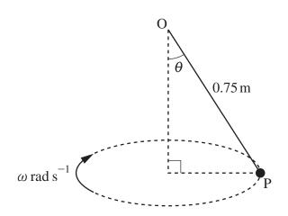
The diagram shows a particle P, of mass 0.2 kg, which is attached by a light inextensible string of length 0.75 m to a fixed point O.
