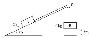
Block A is more than d m from P. The blocks are released from rest and A moves up the ramp. The coefficient of friction between A and the ramp is  $\frac{1}{2\sqrt{3}}$ .
